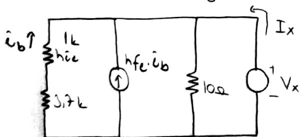
$$R_o = \frac{V_x}{I_x} \quad I_x = \frac{V_x}{3,38k} \quad \boxed{R_o = 3,38k \Omega}$$
