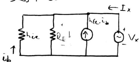
$$I_x + h_{fe} \cdot i_b = \frac{V_x}{R_E} + i_b = 0 \quad i_b = -\frac{V_x}{h_{ie}}$$
