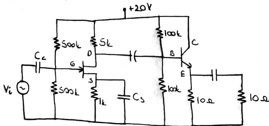
FET;  $g_m = 1 \text{ mS}$ ,  $r_d = 20 \text{ k}\Omega$
